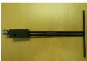
Figure 1 – MVG COMOSAR Validation Dipole
