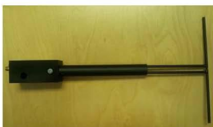
Figure 1 – MVG COMOSAR Validation Dipole
