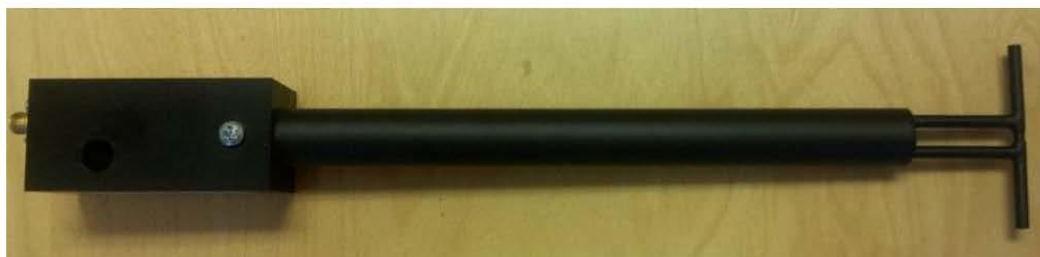
Figure 1 – MVG COMOSAR Validation Dipole
