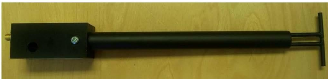
Figure 1 – MVG COMOSAR Validation Dipole
