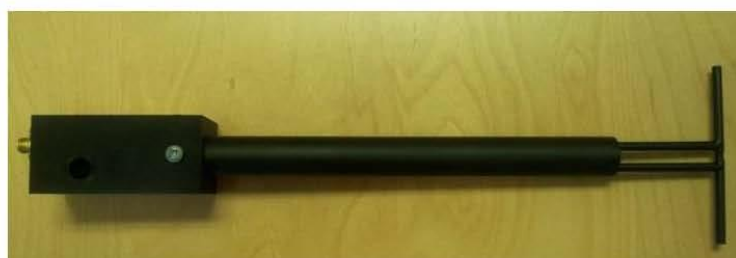
Figure 1 – MVG COMOSAR Validation Dipole
